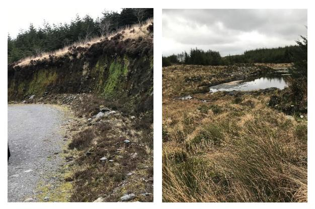
Figure 2-1 Left: Excavation exposing a thin layer of peat over till at proposed T4. Right: Waterlogged peat in the vicinity of the proposed temporary compound.
